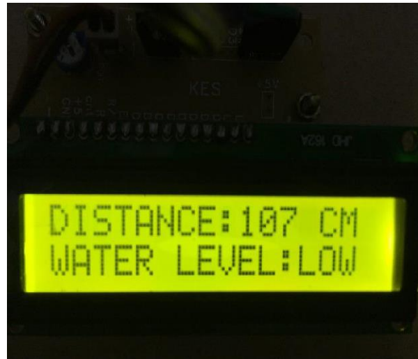
Fig: 4.2 Displaying water level in LCD
